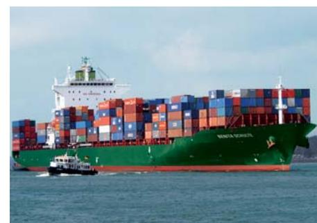
Heavy Industries has, with a length of 260 metres and a breadth of 32,20 metres, a deadweight of 50.500 t. She has a container capacity of 4253 TEU or 2805 TEU with a 14 to. homogenous load, as well as 400 reefer plugs.
